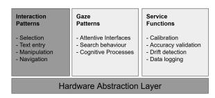
Figure 1: The basic architecture of the EyeMRTK. Focus of this paper are the HAL and the interaction patterns for selection.
